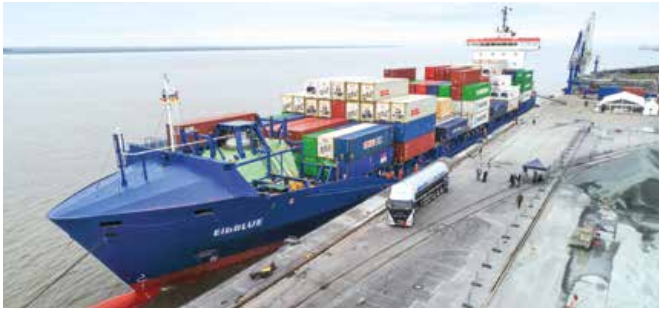
The ElbBlue was the first ship to bunker SNG, generated from renewable energy Source: MAN Energy Solutions
