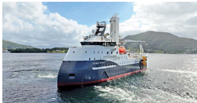
The Ulstein SX222 CSOVs have a length of 89.6m and a beam of 19.2m
