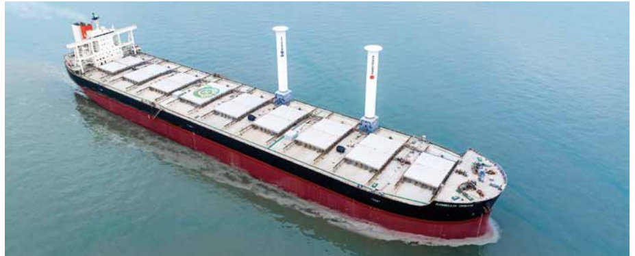
Two Norsepower Rotor Sails™ installed on board bulk carrier Camellia Dream Source: Norsepower
