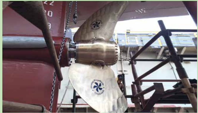
PCP retrofit to Thor R
