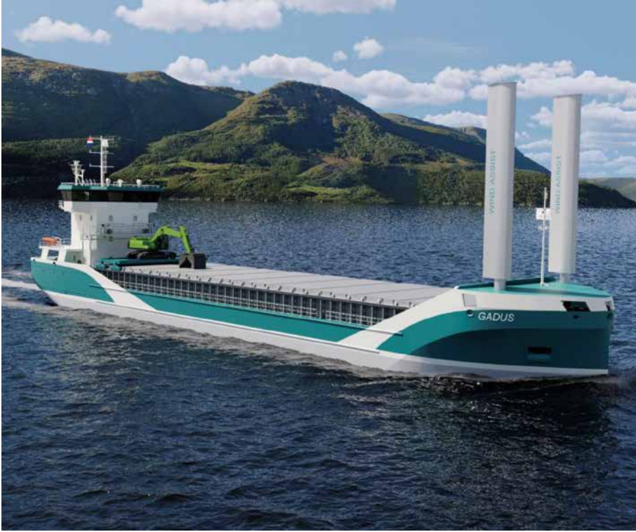
Illustration of the self-discharging 5,600dwt dry cargo vessel
