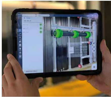
Digitised worker assistance for the installation of pipe supports Source: Sikla GmbH
