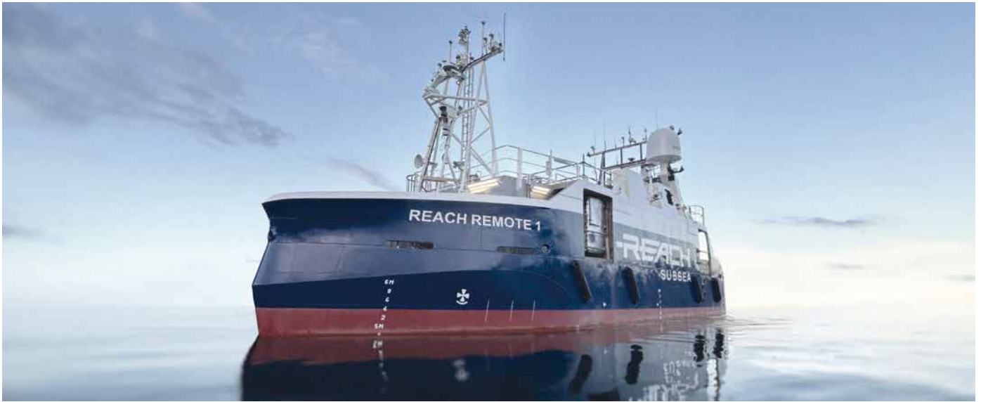
Reach Remote is the first of a pair of unmanned surface vessels for underwater survey projects
